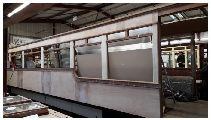
All the insulation cladding is fitted ready for the panels.
